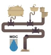
The sewer house connection is the pipe that carries wastewater from your home to the sanitary sewer main located in the street.
