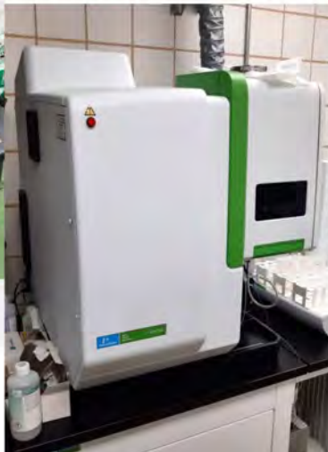
Metals Analysis on the Inductively Coupled Plasma (ICP) Spectrophotometer
