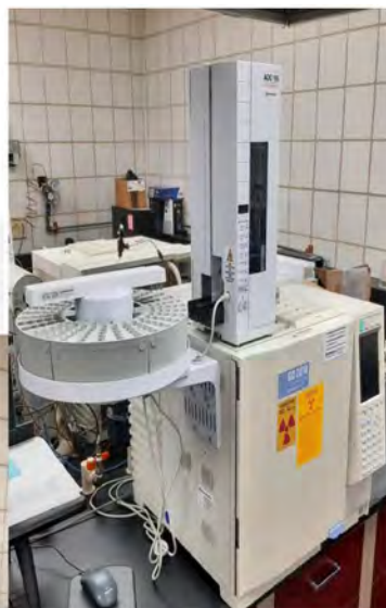
Gas Chromatograph - Electron Capture Device (GC-ECD) for HAAs
