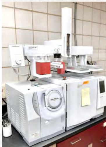
Gas Chromatograph - Mass Spectrometer (GCMS) for Taste & Odor Compounds
