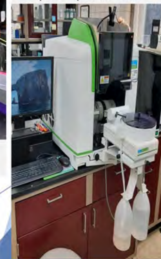
Metals Analysis on the Atomic Adsorption (AA) Spectrophotometer
