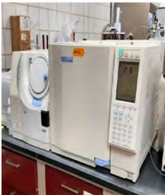
Gas Chromatograph - Mass Spectrometer (GCMS) for THMs & VOCs
