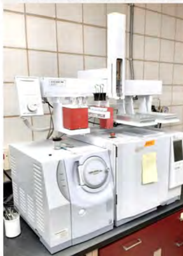
Gas Chromatograph - Mass Spectrometer (GCMS) for Taste & Odor Compounds
