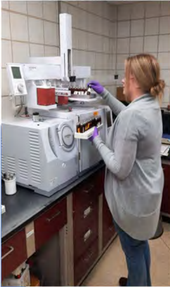
Julie Gillette Loading Taste & Odor Samples on the GCMS
