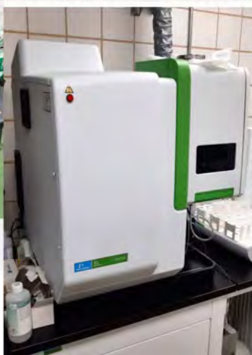
Metals Analysis on the Inductively Coupled Plasma (ICP) Spectrophotometer
