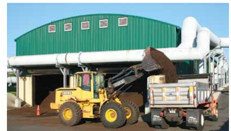
Fairfield—compost loaded onto a truck at the end of the 28-day agitation and aeration period
