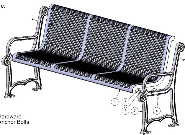
Recommended Surface Mount Hardware: 3/8" x 3-1/2" Concrete Expansion Anchor Bolts (Not Included)
