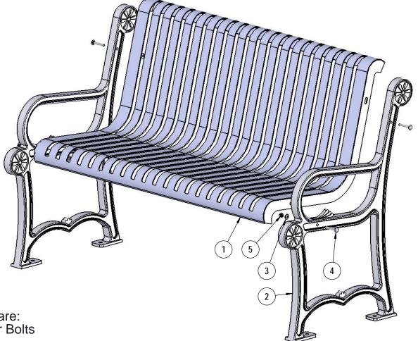
Recommended Surface Mount Hardware: 3/8" x 3-1/2" Concrete Expansion Anchor Bolts (Not Included)
